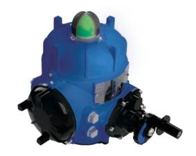
The CEA is equipped with an absolute encoder patterned after the QX encoder, sensing valve position to less than 1.0% in some applications. Valve torque is sensed from motor current, providing a tried and true method of torque control similar to the method use in the QX. The CEA is available for modulating control and can be outfitted with a full suite of network protocols.
