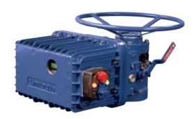
The L120 is factory-lubricated, suitable for weatherproof service in temperatures ranging from -40°C (-40°F) to 65°C (150°F), as well as explosion proof and temporary submersion applications. Weatherproof enclosures meet NEMA 4 standards, as well as NEMA 6, IP67, and IP68 submersible standards. Explosionproof actuators meet Factory Mutual and Canadian Standards Association requirements.
