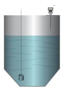
\*Mounting must be electrically connected to tank wall for a single rod probe to work. Dual probe will work without electrical connection.
