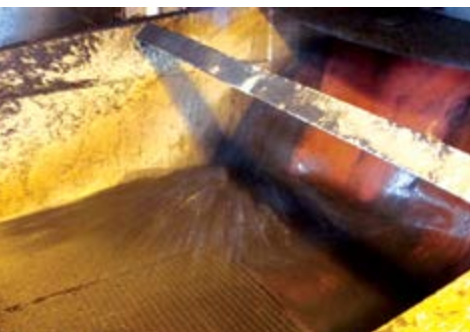
Wet Screens Blocked Chute Detection - Water Sprays
