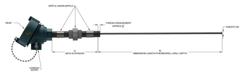
Daily Thermetrics' 310 Series Industrial Sensor Assembly is designed for direct termination into a head via a nipple and union combination. This style can be spring-loaded. This sensor is best suited for use with a thermowell (see Daily Thermetrics' Thermowell Catalog). All aspects of this sensor assembly are customizable, including element type, sheath metallurgy, length, connection type, and head.
