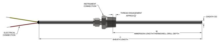
Daily Thermetrics' 210 Series Industrial Sensor is a basic mineral-insulated thermocouple / RTD probe with either bare leads or a connection plug for termination. This sensor is suited for use either in thermowells (see Daily Thermetrics' Thermowell Catalog) or directly in a process. All aspects of this sensor are customizable, including element type, sheath metallurgy, length, connection type, and termination style.
