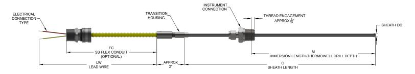
Daily Thermetrics' 220 Series Industrial Sensor with Flexible Leads is a sensor probe with conductor wires that transition into lead wire in flexible conduit for remote termination. This sensor is suited for use either in thermowells (see Daily Thermetrics' Thermowell Catalog) or directly in a process. All aspects of this sensor are customizable, including element type, sheath metallurgy, length, connection type, and termination style.
