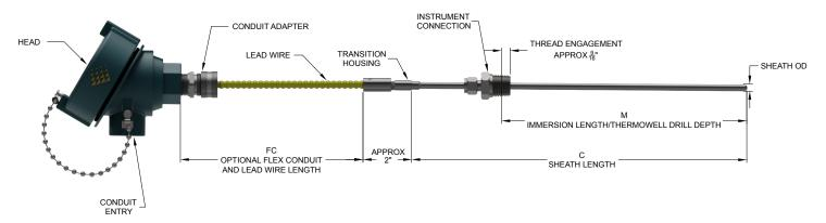
Daily Thermetrics' 360 Series Remote Industrial Sensor Assembly is a sensor probe with conductor wires that transition into lead wire in flexible conduit for remote termination into a head. This sensor is suited for use either in thermowells (see Daily Thermetrics' Thermowell Catalog) or directly in a process. All aspects of this sensor assembly are customizable, including element type, sheath metallurgy, length, connection type, and head.
