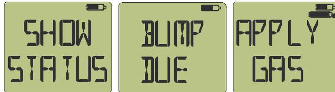
The detector will flash between "BUMP DUE" and "APPLY GAS". Apply gas to the detector's gas inlet. Once all sensors have gone into alarm, the unit will return to normal operation (in alarm) and the bump due date will be reset.
